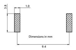
All dimensions in mm Tolerances unless otherwise specified: ±0.20mm
